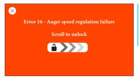
When this message is on screen this means that the product is in blocking mode and you can remove the error. You can do this by swiping to the right in the center of the screen.
